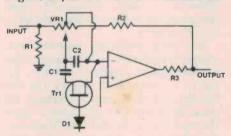
Figure 10. Part of the equalisation circuit of the Teac 35-2B recorder.
