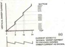
Figure 4c: In this graph the scan lines for each character row are vertically squeezed together to obtain a space between rows. The current to be added to the normal yoke current is shown beneath.
