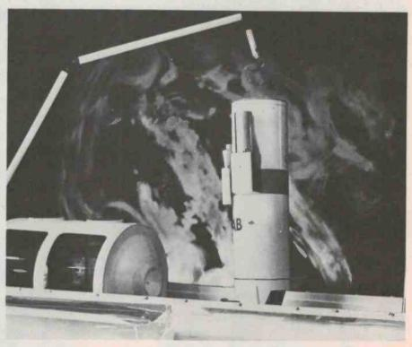
Mock-up model of Starlab being lifted out of the instrument bay of the Space Shuttle.
