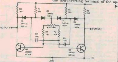
Figure 5b. Improved version of variable M/S ratio astable with waveform correction and sure-start facility.
