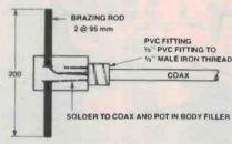
Figure 4. Construction of the dipole.
