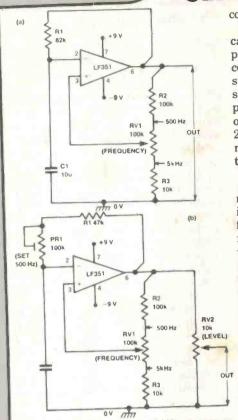
Figure 7. (a) Simple 500 Hz to 5 kHz squarewave generator and (b) an improved version.
