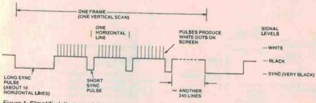
Figure 1: Simplified diagram of the composite video signal.
