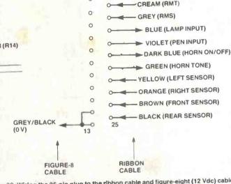
Figure 23. Wiring the 25-pin plug to the ribbon cable and figure-eight (12 Vdc) cable.
