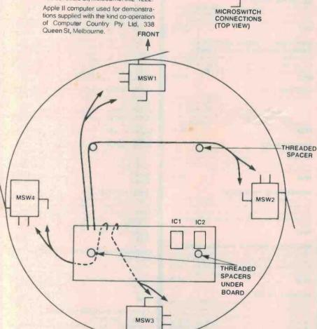
Figure 15. Routing the wires to the sensor microswitches.
