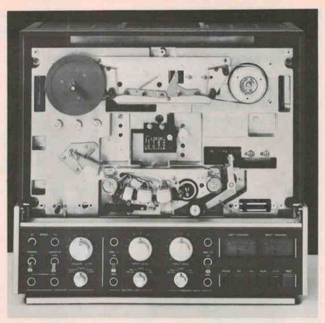
A view of the Revox B77 open-reel deck with the top cover removed to show the tape heads, etc.
