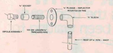
Figure 3. How the antenna support structure is made.
