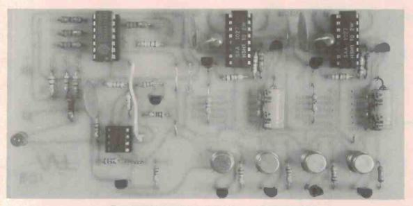
The completed control board, prior to attaching the various cables.
