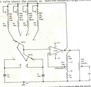
control to a precise minimum value, and Figure 8. Four-decade (2 Hz to 20 kHz) square wave generator. The presets enable the circuit to use a
