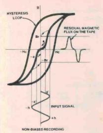
Figure 17. Recording without bias produces severe distortion (Teac).
