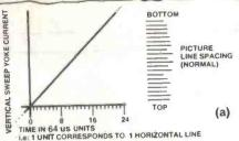
Figure 4a: Graph showing the vertical yoke current during a portion of the sweep. Beside the graph is a representation of the spacing of the scan lines with this normal (unmodified) sweep current.
