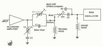
Figure 15. A basic bias oscillator circuit connected to the erase and record heads.
