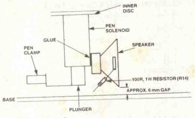
Figure 21. Mounting the speaker:
