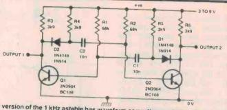
Figure 3. This version of the 1 kHz astable has waveform correction applied via D1 and D2 and produces
