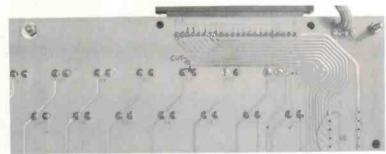
Figure 3. Modifications required to the rear of the keyboard pc board.
