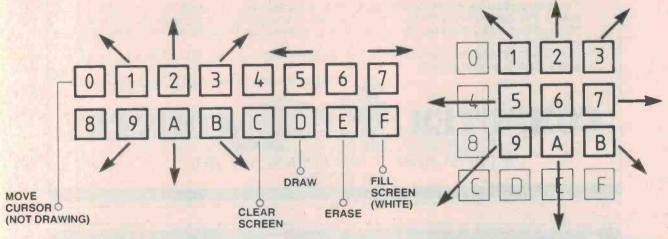
The 'standard' '660 keyboard showing the functions of each key. The heavy arrows indicate which way the cursor moves when you press that key. One press moves the cursor one pixel position.
