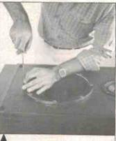
Place and connect the woofer making sure a gasket is in place first. The pic above shows the correct method of "guarding the cone". One hand covers the cone and guides the screwdriver blade. By using this method you can prevent costly damage to your speakers.
