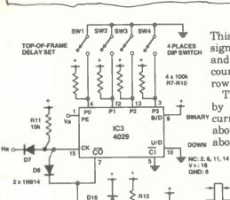
This short pulse, 'T', serves both as the signal to put a space in the display scan. and also presets IC4 again ready to count the lines in the next character
