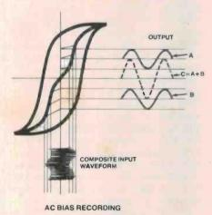
Figure 19. Recording the signal plus blas can produce low distortion (Teac).
