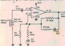
Figure 9. A simple playback amplifier with equalisation (National Semiconductor).
