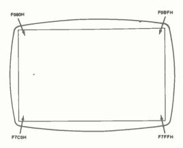
Figure 1. These are the four corner addresses of the screen. Format is 30 lines of 64 characters, so there are 1920 available locations.
