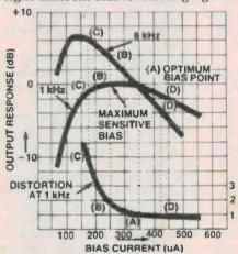
BIAS CURRENT VS. RELATIVE OUTPUT LEVEL/DISTORTION
