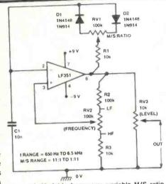
Figure 9. Variable frequency, variable M/S ratio
