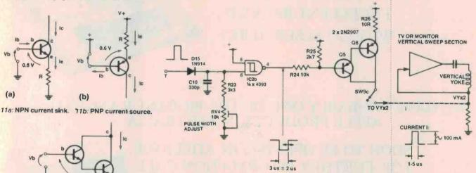
Figure 10: This circuit sends a pulse to the yoke to make the between-row step in the scan occur sharply.
