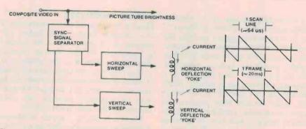
Figure 2: Conceptual picture of TV or monitor sweep sections.
